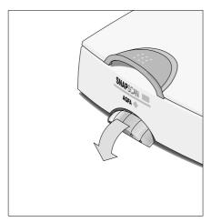
3 Remove the button cap by lifting it at the underside and sliding it out of its lip.
